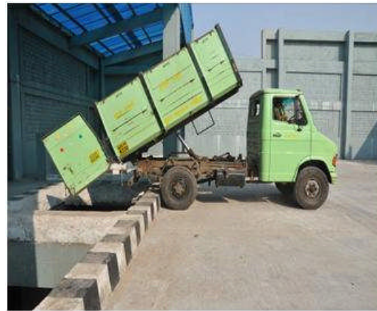
Tipping Platform at Surat Transfer Station
